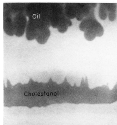
Fig. 2. Separation of paraffin oil from cholesterol in reversed-phase system. Kieselguhr, developed twice in n -heptane at room temperature.
